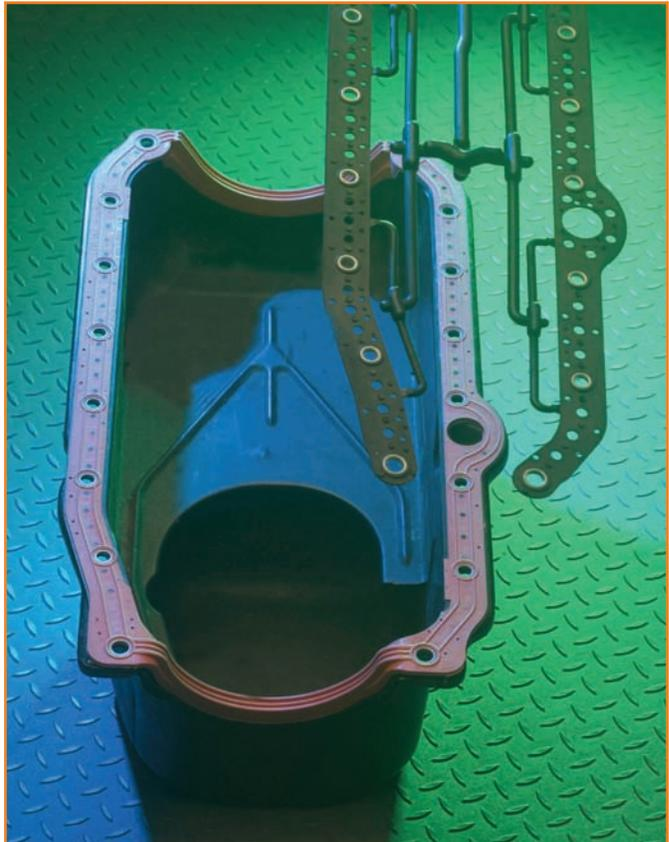
duced from the 2-cavity parting-line injection mold had plastic flashing through only some of the holes within the part. The holes, approximately 1/8" in diameter, that displayed the problematic flashing were mainly in the area of the part closest to the injection nozzle. Although the gates feeding each cavity were evenly spaced and geometrically bal-
