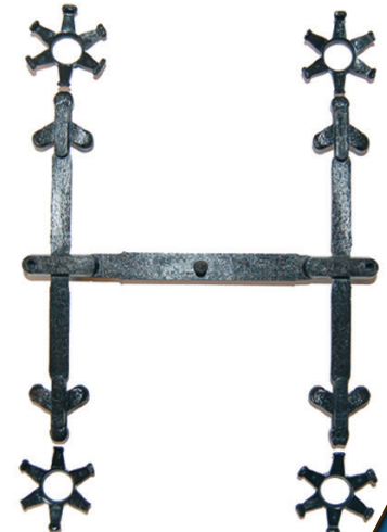
Uniform filling after MeltFlipper®
