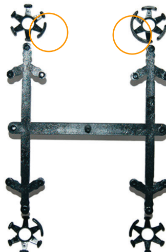
Filling imbalance due to shear
