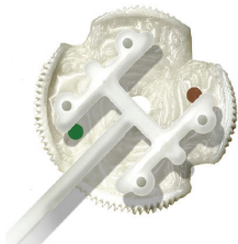
Fig 1: Conventional Asymmetrical Fill Pattern
