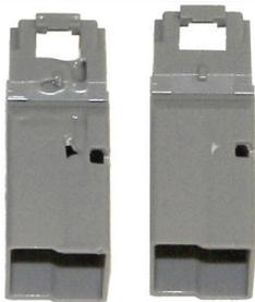
Figure 1: Conventional fill pattern and resulting gas trap
