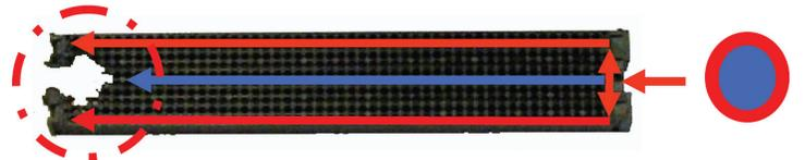
Figure 1: Backfilling condition due to conventional filling pattern
