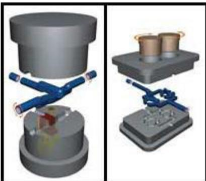
Brand-new iMARC systems will take the MeltFlipper and MAX technologies a step further, turning them into adjustable inserts so that flow in the runner and cavity can be fine-tuned by the user. Since iMARC systems are based on MeltFlipper and MAX technologies, they fall into two primary categories—adjustable single-axis and adjustable multi-axis control systems.
