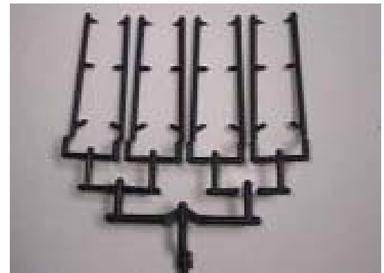
Figure 2: After photo showing the MeltFlipper runner system used to balance the material properties to and within the cavities.
