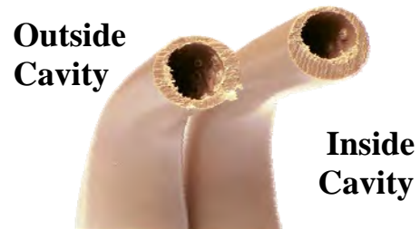
Figure 2: Part cross-sections illustrating the gas channel differences between the inside cavities versus the outside cavities.
