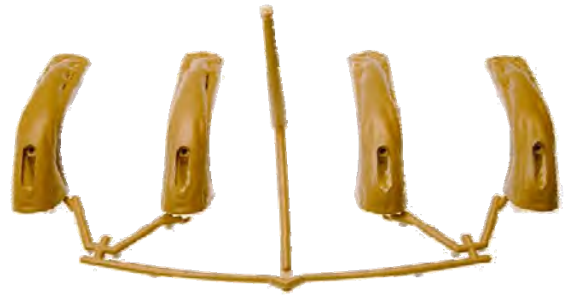
Figure 3: Short shot results after the MeltFlipper technology was applied, showing all cavities filling uniformly.
