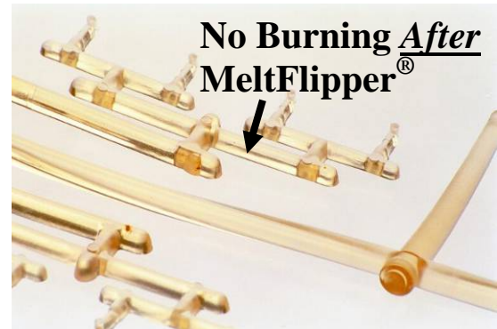
Figure 3: Illustration showing how the MeltFlipper technology eliminated the material degradation due to shear burning in a 32-cavity flexible PVC mold.
