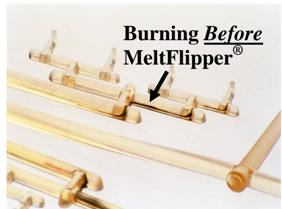
Figure 2: Illustration showing material degradation due to shear burning in a 32-cavity flexible PVC mold.
