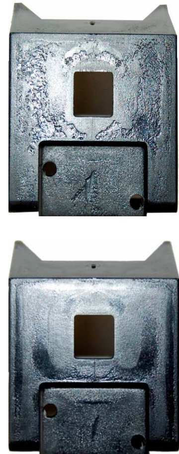
Figure 1: Top - Cosmetic blemishes on the top surface with conventional runner system.
