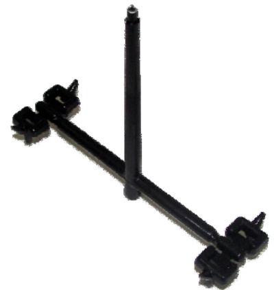
Figure 3: Runner system for the 4 cavity cord tilt housing
