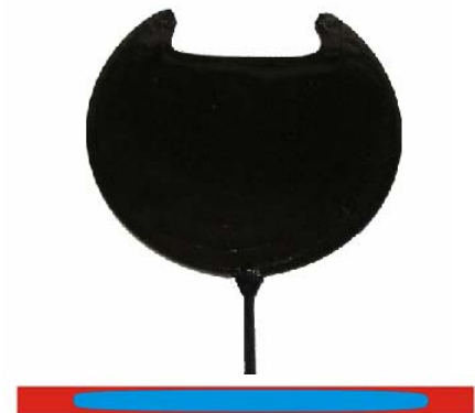
Figure 2: Filling pattern in a single cavity disk without MeltFlipper MAX.
