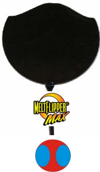
Figure 4: Filling pattern in a single cavity disk achieved with MeltFlipper MAX.
