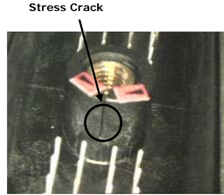
Figure 2: Assembled component with stress crack
